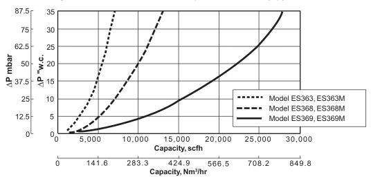
Figure 3.2. Flow vs Pressure Drop, 1-1/2", 2" & 3" NPT (Rp) Models
