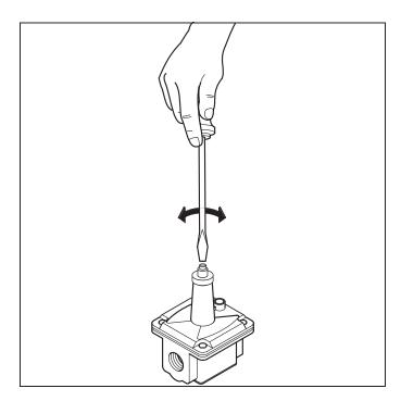
Figure 5.1. Adjustment of Outlet Pressure
