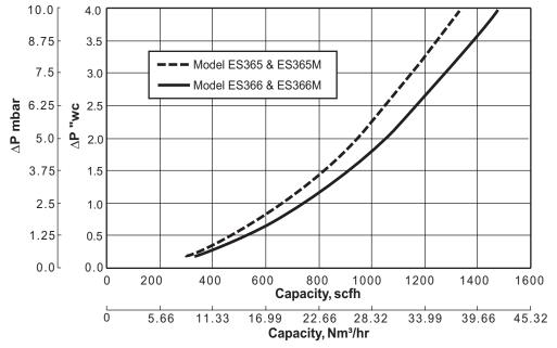
Figure 3.1. Flow vs Pressure Drop, 3/4" & 1" NPT (Rp) Models
