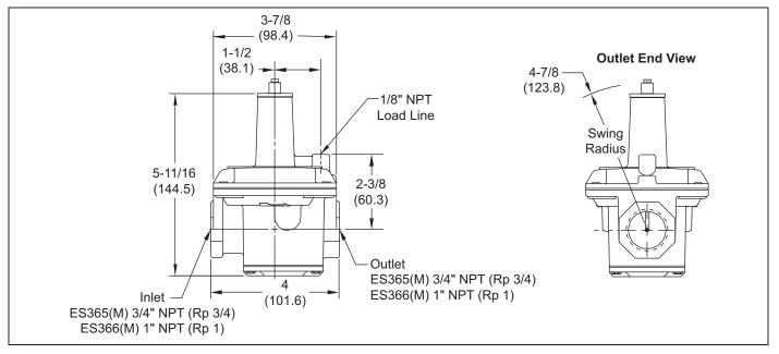
Figure 3.3. Dimensions in inches (mm), Models ES365 (M) & ES366 (M)
